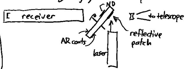
Now the laser does not go through the rotating mirror, eliminating one high-power surface with scatterers. Furthermore, the receiver is better isolated from the beam due to the highly reflective surface.
