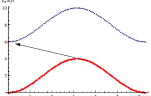
This costs energy  $\Delta E = \epsilon - 4t$  which is finite even as  $N \to \infty$ . A system of fermions with completely filled bands describes an insulator (aka semiconductor). It has an energy gap: the energy of the first excited state is above the ground state energy (even as  $N \to \infty$ ). It is hard to excite.
