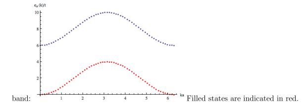
The lowest energy excitation of this system is achieved by taking one of the electrons out of a filled state in the bottom band and raising it all the way to the empty *conduction* band:
