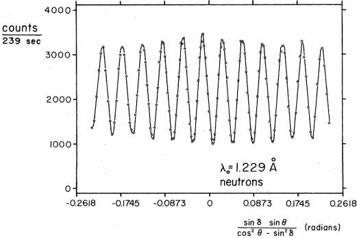
FIG. 7. Example of data obtained by rotating an Si slab in the interferometer (Fig. 6). The counts in detector  $C_3$  are shown. 1/31/2014
