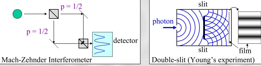
Interference is the hallmark of quantum mechanics
