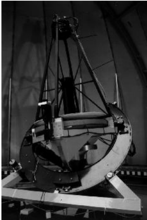
Fig. 15.— Token space filler, (not directly related to PSF photometry): The 76 cm Katzman Automatic Imaging Telescope (KAIT) located at Lick Observatory. The world's most successful low z supernova search telescope, and the ultimate source of nearly all of your photometric data.
