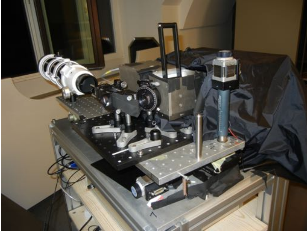
Entangled photon receiver and polarization analyzer
