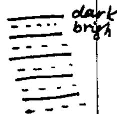
\* If the glass plates are not exactly flat at the order of light wavelength, the pattern will not be straight lines. Similarly, if the lens is not spherical, the Newton rings will not be circular — precision measurement
