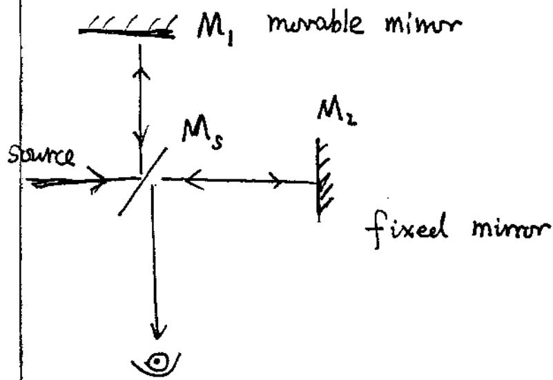
a movement of  $M_1$  at  $\frac{\lambda}{4}$ , produces a light distance difference of  $\frac{\lambda}{2}$ , change constructive  $\leftrightarrow$  destructive interference
