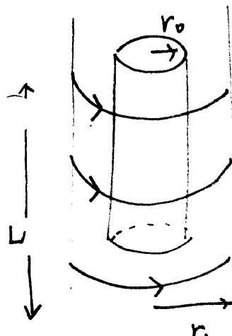
long cylinder: sample in a solenoid
