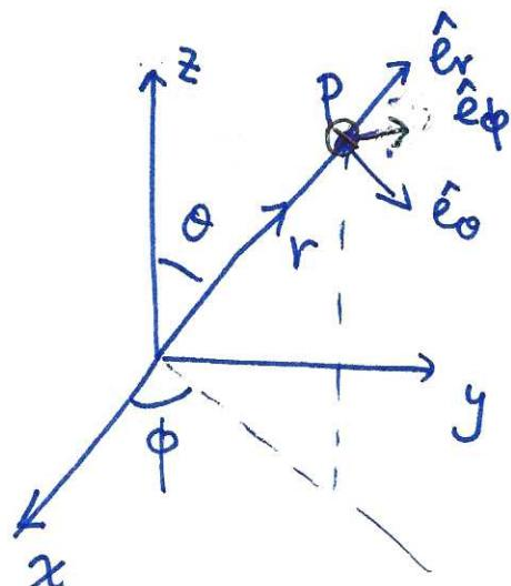
$$\begin{aligned}\hat{e}_r &= \begin{pmatrix} \sin\theta \cos\phi & \sin\theta \sin\phi & \cos\theta \\ \cos\theta \cos\phi & \cos\theta \sin\phi & -\sin\theta \\ -\sin\phi & \cos\phi & 0 \end{pmatrix} \begin{pmatrix} \hat{x} \\ \hat{y} \\ \hat{z} \end{pmatrix} \\ \hat{e}_\theta &= \\ \hat{e}_\phi &= \end{aligned}$$
