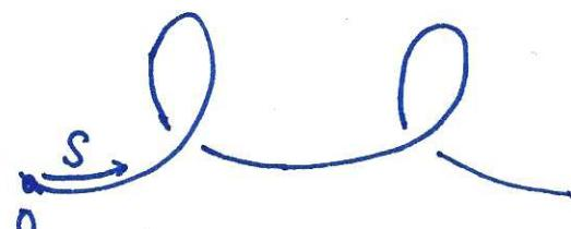
Since the motion is constrained along the curve, — the direction of the velocity is along the tangential direction  $\vec{t}_t$ , and the speed is simply  $\dot{S}$ .  $\Rightarrow \vec{v}(S) = \dot{S} \vec{t}_t(S)$
