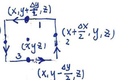
$$\int_1 + \int_3 = -\Delta x \cdot \left[ F_x(x, y + \frac{\Delta y}{2}, z) - F_x(x, y - \frac{\Delta y}{2}, z) \right]$$
