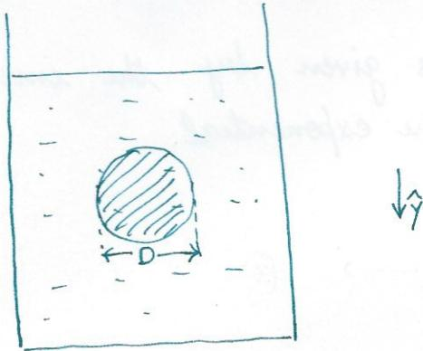
$D$ : diameter of ball $\rho_s$ : density of ball $V$ : volume of ball $\rho_g$ : density of glycerine $\eta$ : viscosity of glycerine $F_B$ : Buoyant force on the ball $f_{lin}$ : linear drag on ball $v(t)$ : velocity of ball at time  $t$  $v_\infty$ : terminal velocity of ball $m$ : mass of ball
