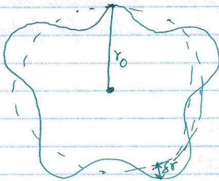
If  $r$  is the distance between the particles, we define  $\delta r = r - r_0$  as the deviation of the distance from the equilibrium distance  $r_0$ .
