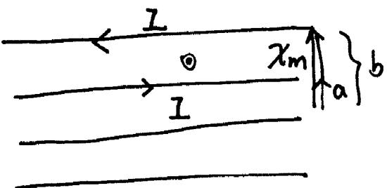
$$\vec{M} = \chi_m \vec{H} = \frac{2\chi_m I}{sc} \hat{e}_\phi \Rightarrow \vec{J}_b = c \nabla \times \vec{M} = \frac{1}{s} \frac{\partial}{\partial s} \left( s \frac{2\chi_m I}{s} \right) \hat{z} = 0$$
