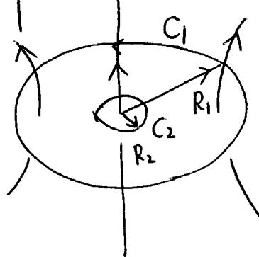
$$B_1 = \frac{2\pi I_1}{CR_1}, \quad \Phi_{21} = \pi R_2^2 \frac{2\pi I_1}{CR_1} = \frac{2\pi^2 I_1 R_2^2}{CR_1}$$
