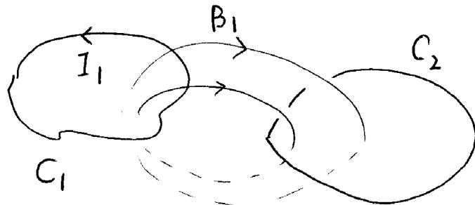
flux from  $I_1$  through loop  $C_2$
