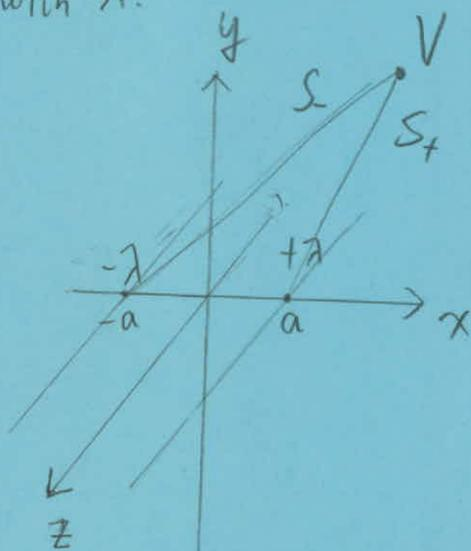
$$S_+ = \sqrt{(x-a)^2 + y^2} \quad \text{and} \quad S_- = \sqrt{(x+a)^2 + y^2}$$
