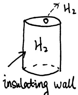
$H_2$  leaks out of the hole. If proton and electron charges are not exactly cancelled, the leaking of  $H_2$  atom will change the total charge and its electric potential.  $\Rightarrow < 10^{-20} e$
